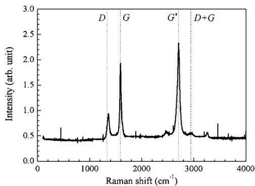
Fig. 7. Raman spectra of CNB formed from arc soot annealed in Ar at 2800°C.
