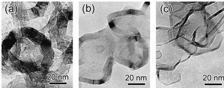
Fig. 8. TEM images of CNB oxidized in air for 15 min at (a) 600, (b) 625 and (c) 650°C.
