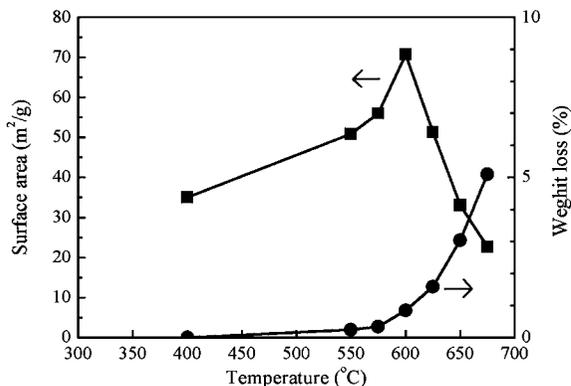
Fig. 10. Surface area changes and weight loss of CNB after oxidation in air for 1 h at different temperatures. ( ) Weight loss and ( ) change in surface area.
