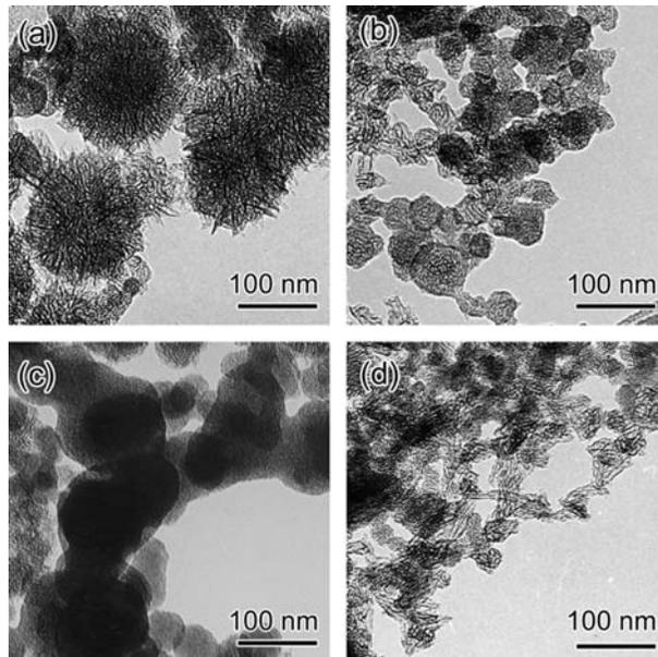
Fig. 2. TEM images of as-prepared arc soot. (a) Graphite spheres with horned surface, (b) graphite spheres without horned surface, (c) amorphous spheres, and (d) structures other than spheres.
