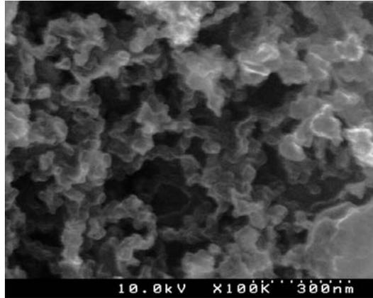
Fig. 4. FE-SEM image of CNBs from arc soot heated at 2800°C in Ar.
