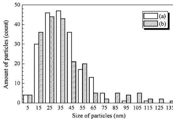
Fig. 5. Size distributions of first-order particles observed by FE-SEM for as-prepared arc soot (a) and CNBs (b) from arc soot heated at 2800°C in Ar.
