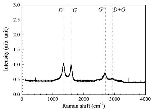
Fig. 3. Raman spectra of as-prepared arc soot.
