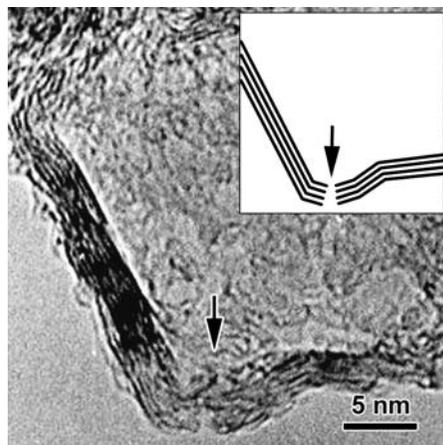
Fig. 9. Magnified TEM image of CNB oxidized at 625°C for 15 min in air. The insert illustrates the pinhole formed at a connection point of the graphite sheets of the balloon shell.
