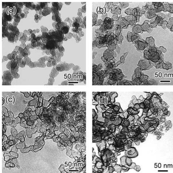
Fig. 6. TEM images of arc soot heated in Ar for 30 min at (a) 1600, (b) 2000, (c) 2400 and (d) 2800°C.
