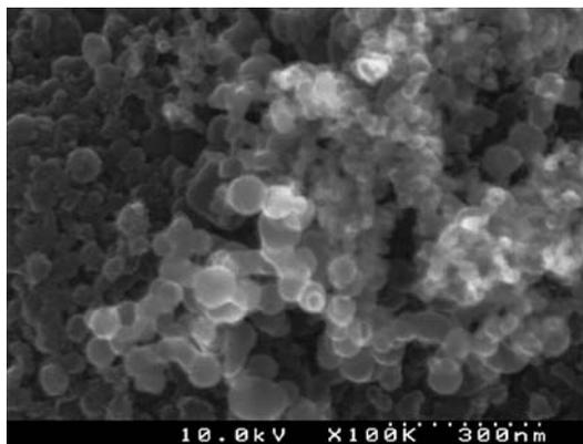
Fig. 1. FE-SEM image of as-prepared arc soot.
