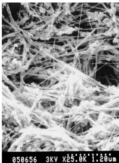
Fig. 4. SEM micrograph of MWNTs and nanoparticles produced in He ( 2.66 \times 10^4 Pa). (15)
