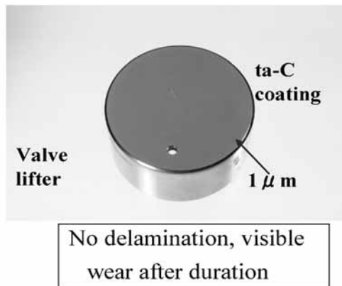
Fig. 12. ta-C coating applied to gasoline engine valve lifter.
