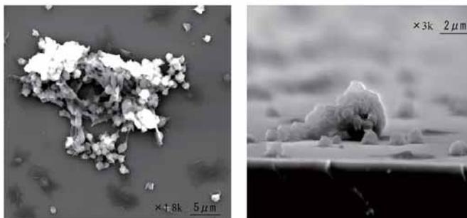
Fig. 2. SEM images of thrombus formation on the substrate (SUS 316L). Local platelet activation promotes the recruitment of platelets and the formation of thrombus.
