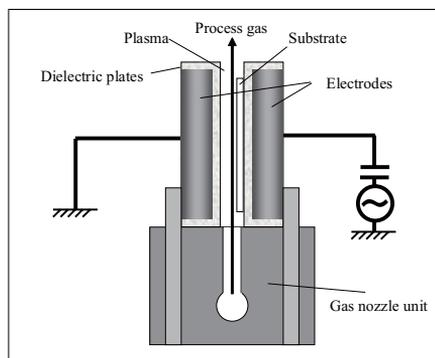
Fig. 5. Schematic diagram of APG plasma CVD equipment. Plasma is sustained between parallel-plate electrodes covered with a dielectric plate.
