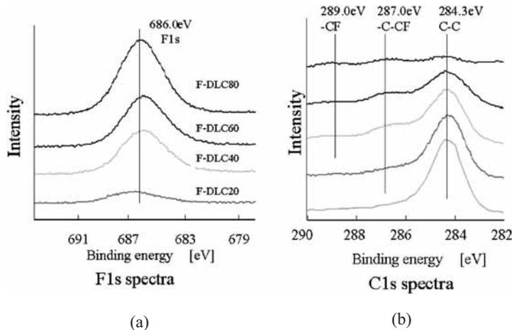
Fig. 1. XPS spectra of DLC, F-DLC20, F-DLC40, F-DLC60 and F-DLC80. (a) F1s XPS. (b) C1s XPS.
