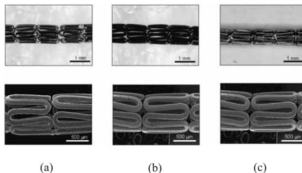
Fig. 4. Availability of DLC and F-DLC films on commercially available coronary stents. (a) Uncoated stainless-steel stent (GFXII, S670, Medtronic Inc., MN, USA). (b) DLC-coated stent. (c) F-DLC-coated stent. Macroscopic findings (upper case) and SEM findings (lower case) of these stents were observed. The surfaces of coated stents were smooth without any cracking of the films.
